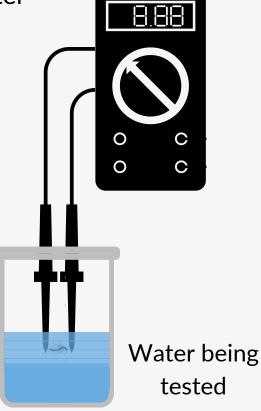
The conductivity probe measures the **resistance** met by the electrical current.
