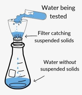
**Then**, the filter that caught the sample's suspended solids is dried. This is to get rid of the water weight — the solids, not the water, are the target of this test.
