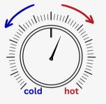
When the thermometer probe is in contact with something **hot**, the more sensitive metal expands, making it longer than the other metal. This pulls the strip on the dial toward the right, **indicating a higher temperature**.
