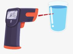
Instead, a "laser thermometer" measures using the infrared light emitted by the object being measured. The infrared wavelength an object emits corresponds to its temperature. The thermometer calculates and displays the temperature of the object.
